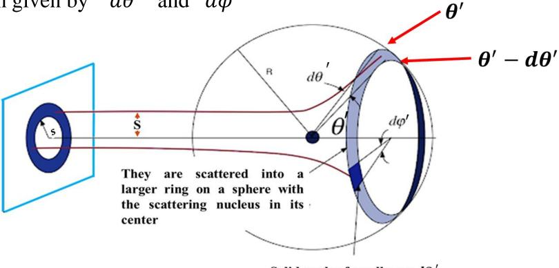
The No. of scattered particles in solid angle " $d\Omega'$ " will be proportional to the intensity of the incident particles and the magnitude of solid angle
